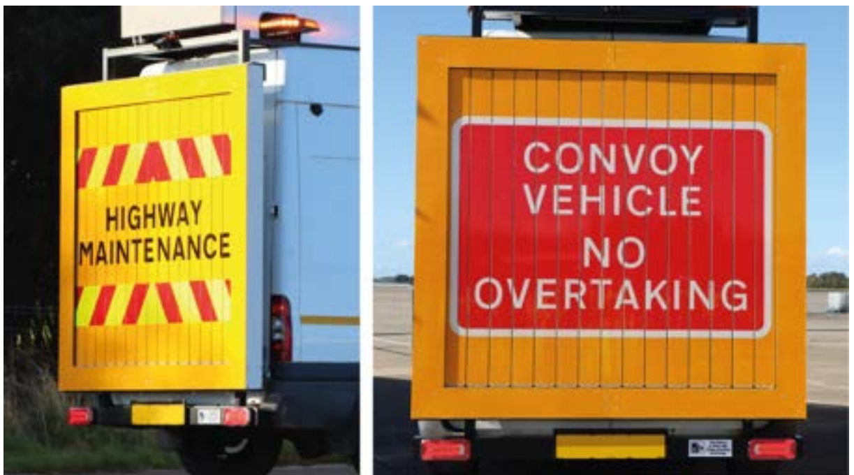
Figure A.10 Rear of enhanced mobile carriageway closure trial vehicle lower panel
